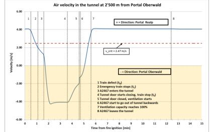
INVESTIGATING DIFFERENT OPERATIONAL SCENARIOS FOR THE PROPOSED EMERGENCY VENTILATION SYSTEM IN FURKA TUNNEL
