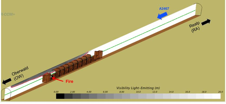
INVESTIGATING DIFFERENT OPERATIONAL SCENARIOS FOR THE PROPOSED EMERGENCY VENTILATION SYSTEM IN FURKA TUNNEL
