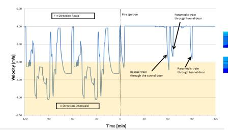
INVESTIGATING DIFFERENT OPERATIONAL SCENARIOS FOR THE PROPOSED EMERGENCY VENTILATION SYSTEM IN FURKA TUNNEL
