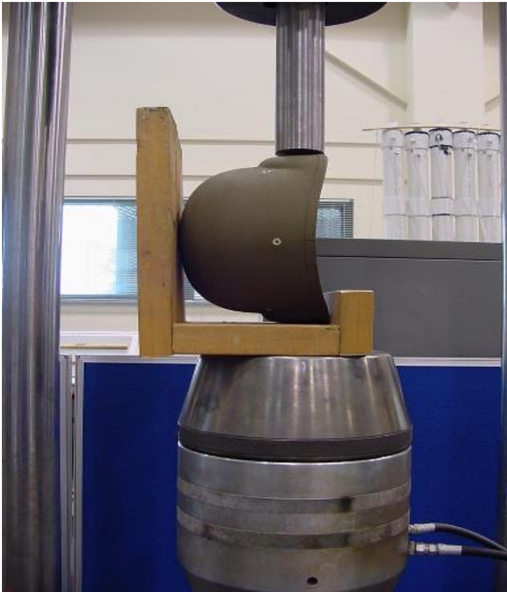
FIGURE 5. Jig – Side to side compression resistance.
