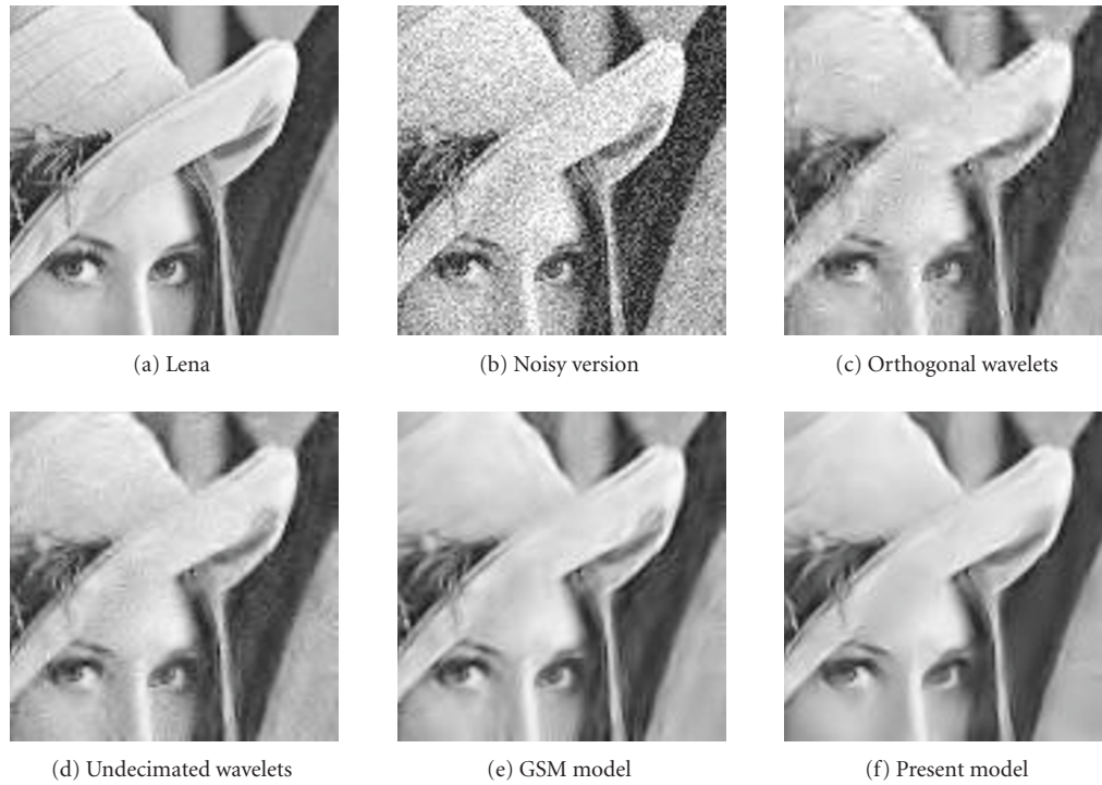
FIGURE 13: Denoising results with Lena image at medium noise level. (a) 112 \times 112 detail of the image “Lena.” (b) Same image corrupted by Gaussian noise for a PSNR of 20.22 dB. (c) After denoising using orthogonal wavelets a high level of artifacts appears. (d) The quantity and strength of artifacts is reduced thanks to the use of undecimated wavelets. (e) The GSM model allows an additional reduction of the number of artifacts. (f) The proposed model also allows to reduce the appearance of artifacts, preserving particularly smooth gradients of luminance. Nevertheless the model shows difficulties in capturing some intricate features in particular close to junctions (see, e.g., the right eye) and to adjacent parallel lines (e.g., upper end of the hat border).
