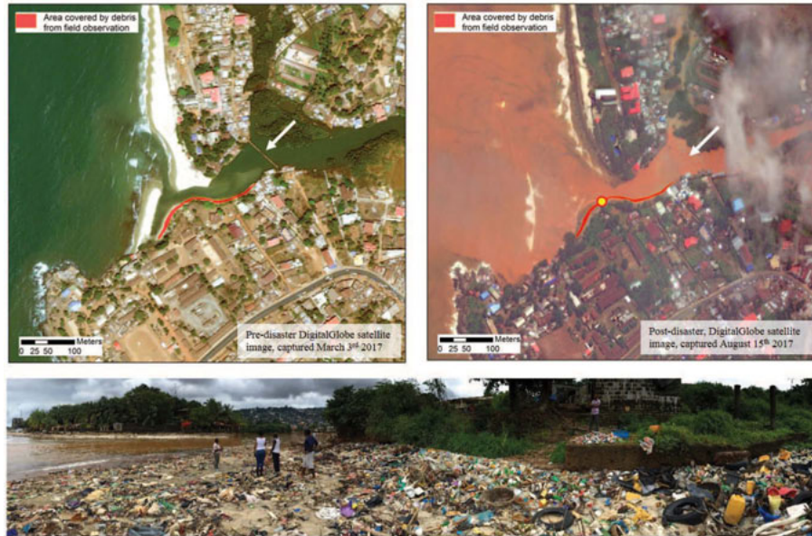
FIGURE 38: Debris at Lumley Creek Resulting from Flooding and Debris Flow Related to Regent Landslide Disaster
