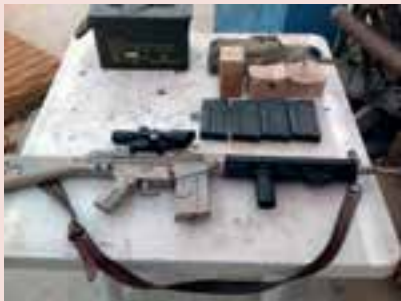
Photo A23 A G3A3-pattern self-loading rifle. Note the after-market optical sight, railed fore-end, and custom paint finish
