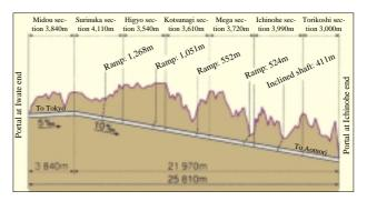
Fig. 3 Longitudinal section of tunnel showing construction sections
