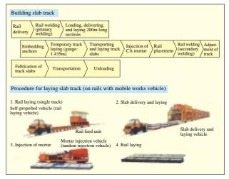
Fig. 7 Procedure for laying track for the Morioka-Hachinohe section of the Tohoku Shinkansen
