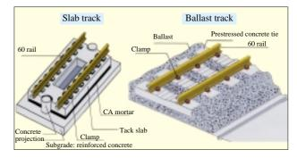
Fig. 8 Slab track and ballasted track
