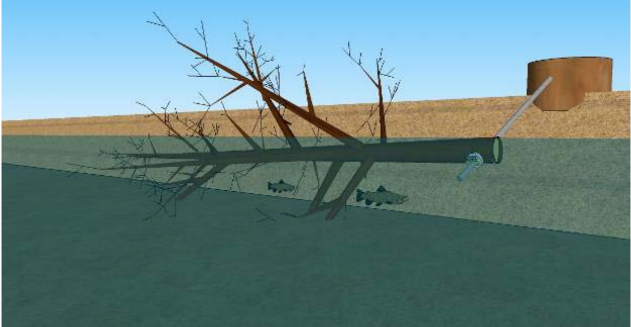
Figure 6 Schematic of tree anchored by cable to its stump
