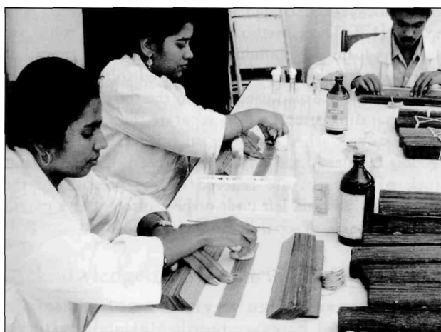
Cleaning and imparting flexibility to palm leaves using oils, moisture and solvents carry inherent risks
