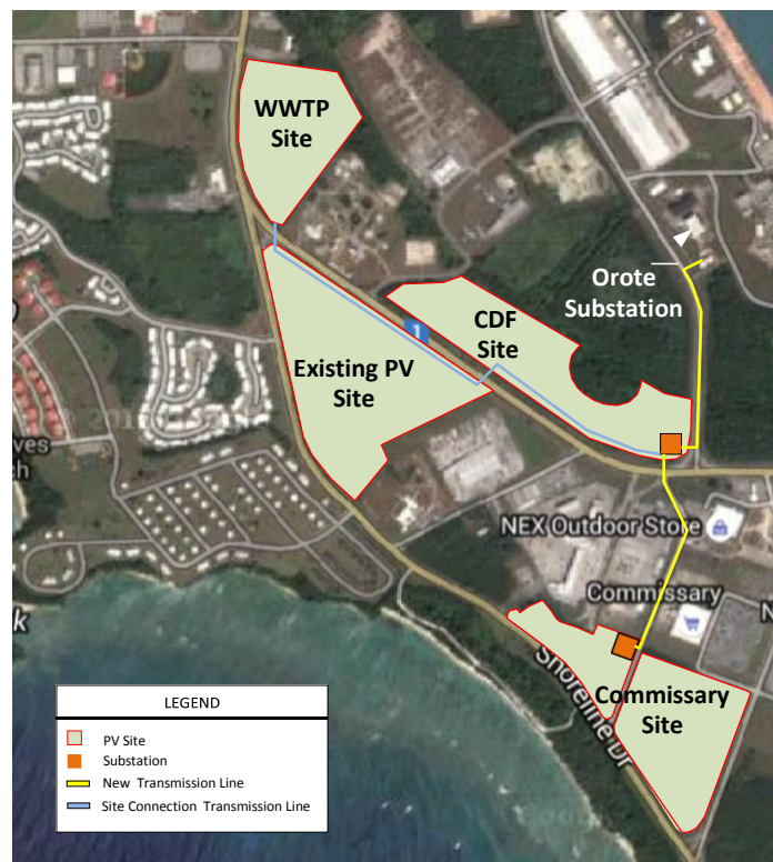
Figure 2 – Naval Base Guam Sites Interconnection
