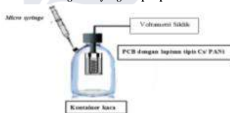
Gambar. Rangkaian pengujian gas \text{NH}_3 berbasis CS/PANi
