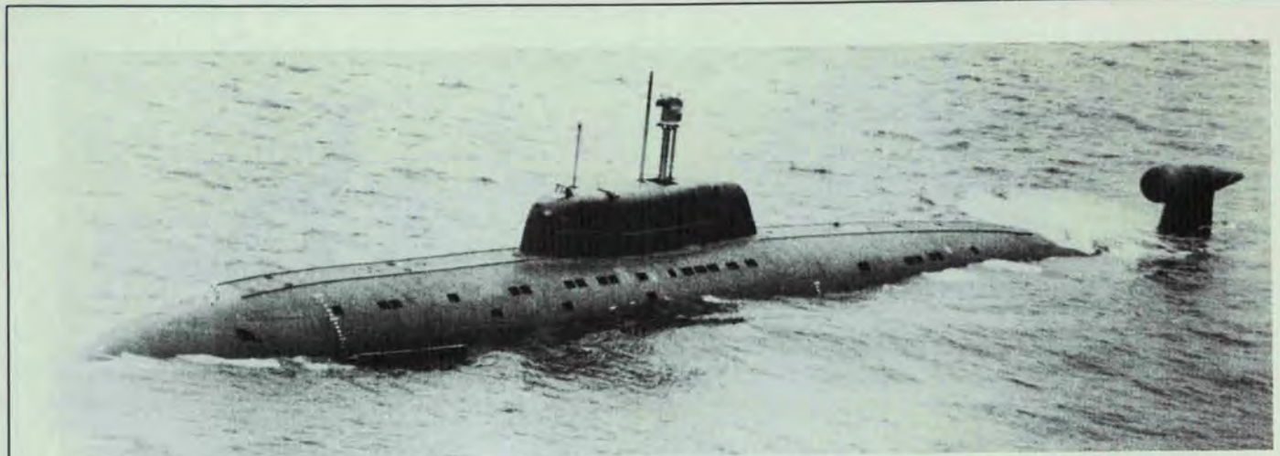
The new SIERRA-Class nuclear-powered attack submarine, with a stern-mounted towed-array sonar pod, became operational in 1984.
