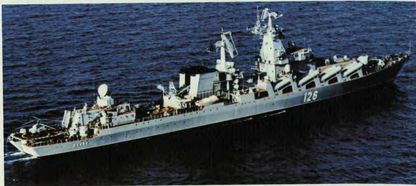
The SLAVA-Class guided-missile cruiser carries sixteen, 550-kilometer antiship cruise missiles as well as air- and point-defense missiles and a 130-mm twin-barrel gun.
