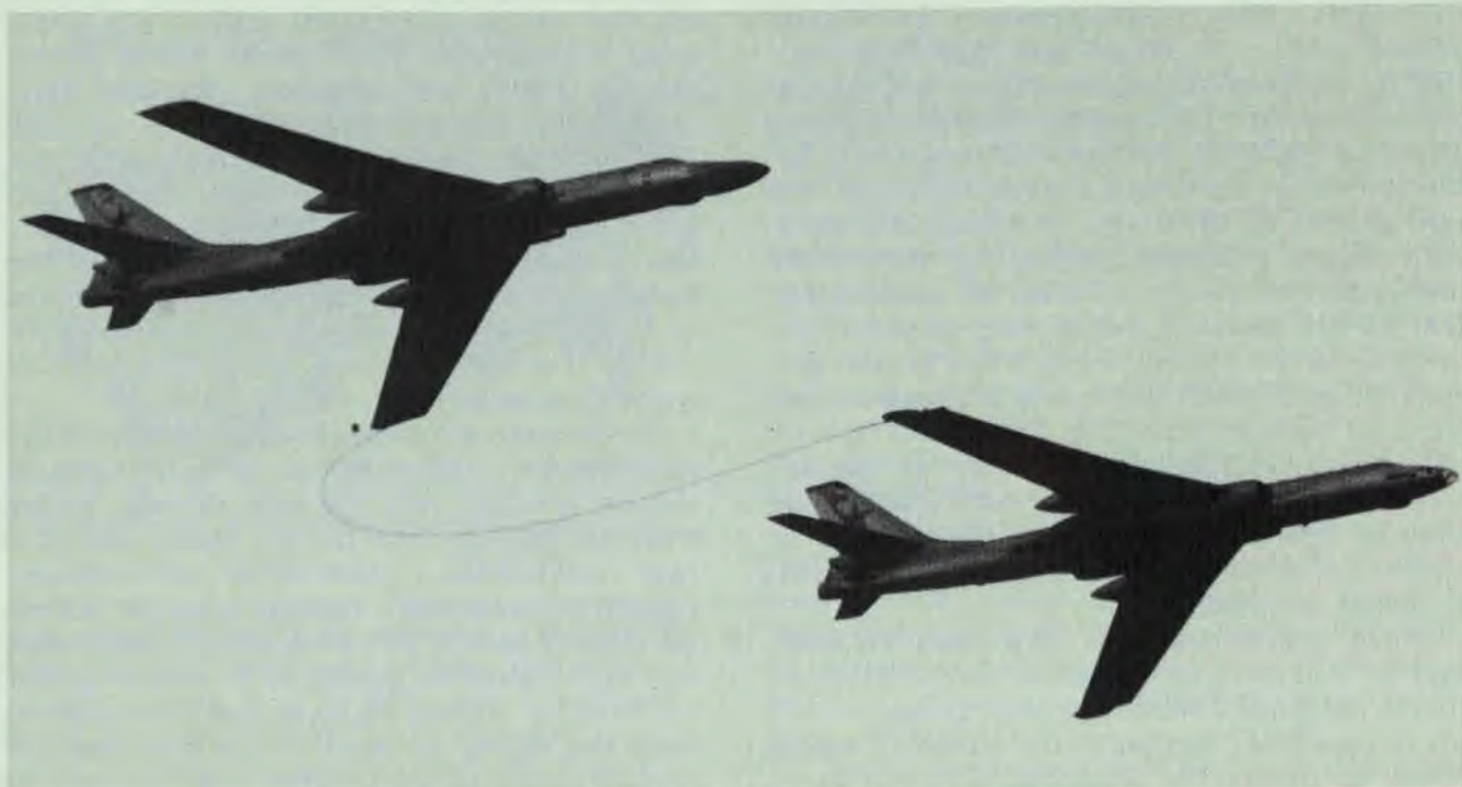
In-flight refueling from BADGER A tankers extends the range of BADGER C strike aircraft.
