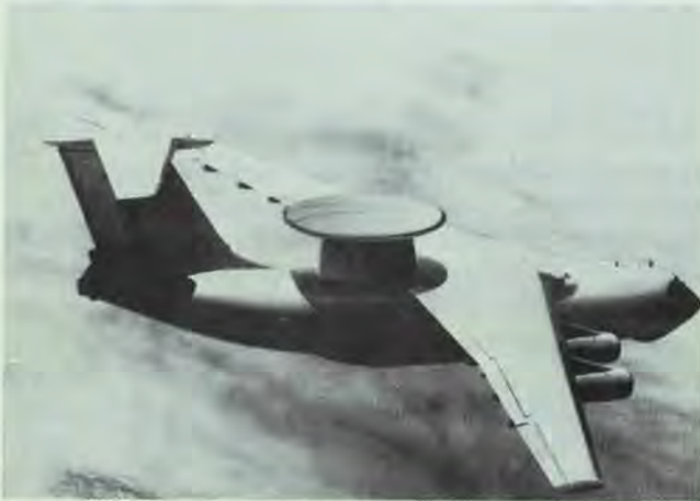
The new Il-76/MAINSTAY aircraft is illustrated as configured for its airborne warning and control mission.
