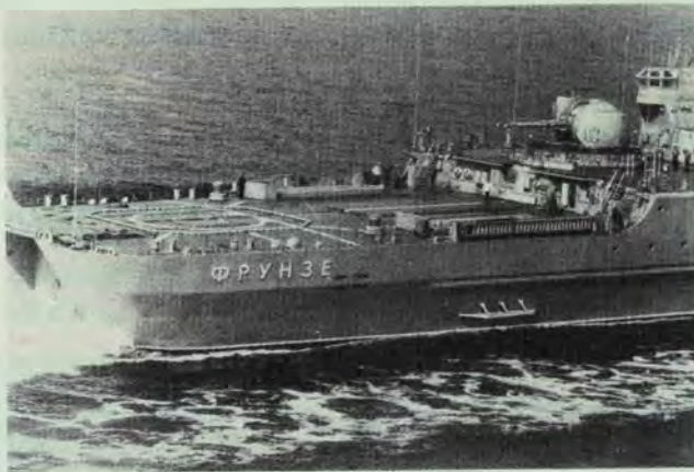
The nuclear-powered guided-missile cruiser FRUNZE, second unit of the KIROV-Class, at 28,000-tons displacement, is 248 meters in length, carries RBU-6000 rocket/launchers, 96 vertically launched SA-N-6 surface-to-air missiles, and 20 SS-N-19 surface-to-surface missiles as well as ADMG Gatling guns on its foredeck (facing page). Its radars and electronic warfare suite contribute to its surface strike and fleet defense missions. Its afterdeck has a twin-barrel 130-mm gun, landing platform and handling facilities for embarked HELIX helicopters.
