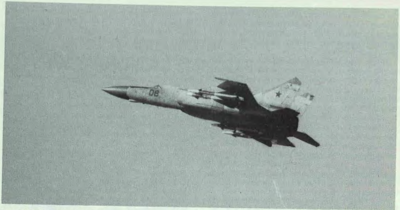
The MiG-25/FOXBAT E interceptor, above, has a limited look-down/shoot-down capability. Acquisition of Western technology enabled the USSR to fit the MiG-31/FOXHOUD interceptor with a true look-down/shoot-down radar system.
