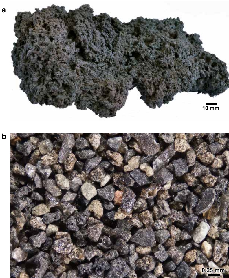
Fig. 2 - Comparison of the material properties of subglacial and subaerial eruption products from the 2010 volcanic eruptions in Iceland. Although the magmatic composition of both eruption products was roughly similar, the scale and properties of the formed materials are clearly different due to the eruption environments. Scoria from the Magni crater (a) illustrates the type of material formed by a subaerial eruption. Ash from the subglacial Eyjafjallajökull eruption (b) shows the end-product of explosive fragmentation and rapid quenching. Scoria samples were collected by the author in 2011 while ash samples were collected by L. Kerstens near Hvosvöller and Mulakot (along the F261 road) four months after the main eruption phase of the Eyjafjallajökull eruption.
