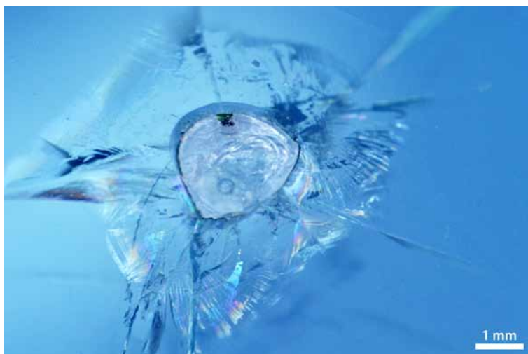
Fig. 23 - The abrasion of the particle surface by impacts of angular grains in many ways resembles the damage caused by stones hitting the windshield of a car, as shown in this image. In amorphous materials such as glass, these 'Boussinesq' crack features are common at all scales of glass fracturing. Clearly visible are lenticular cracks radiating away from the impact point and lateral pseudo-conchoidal fractures where small chips of glass have been removed or are prone to removal by ice infiltration. (Windshield courtesy of W. and N. Remijn)
