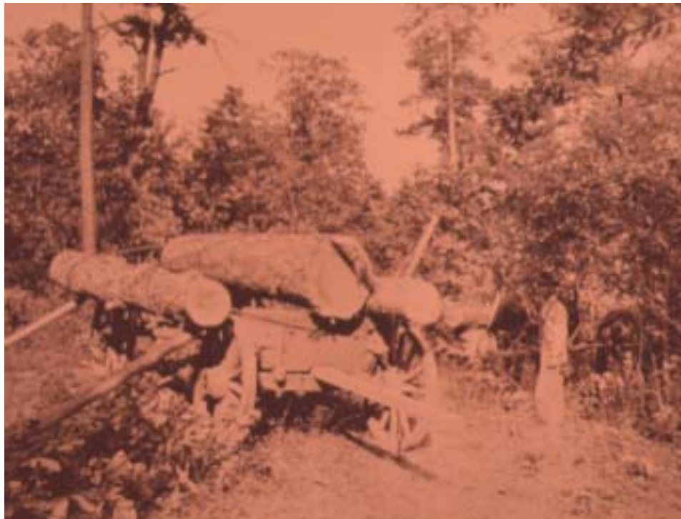
Loading logs by means of cross haul, 1924, Cold Springs Ranger District, Arkansas National Forest. Courtesy of Arkansas History Commission
