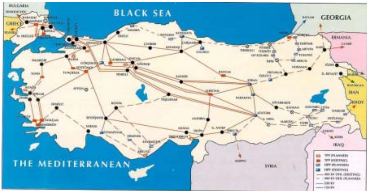
Figure 6.1. Transmission network of Turkey
