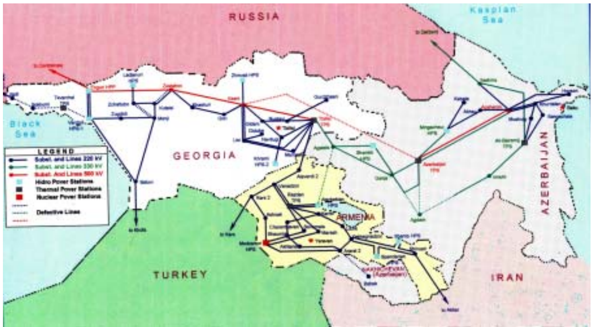
Figure 6.3. Trans-Caucasian Power System
