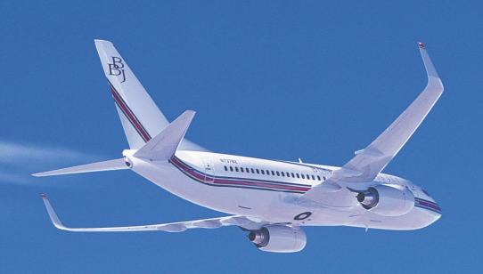
oeing offers blended winglets — upward-swept extensions to airplane wings — as standard equipment on its Boeing Business Jet (BBJ) and as optional equipment on its 737-800 commercial airplane. Winglets also are available for retrofit on in-service airplanes. The 8-ft, carbon graphite winglets allow an airplane to extend its range, carry as much as 6,000 lb more payload from takeoff-limited airports, and save on fuel.
