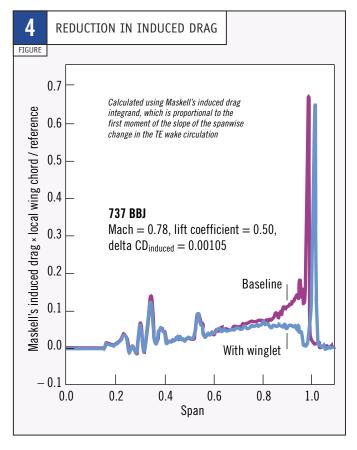
winglet-induced load increase and its distribution along the wing can significantly affect the cost of modifying the wing structure. From the perspective of loads and dynamics, the three areas that affect structural change are static loads, dynamic flight loads, and flutter.
