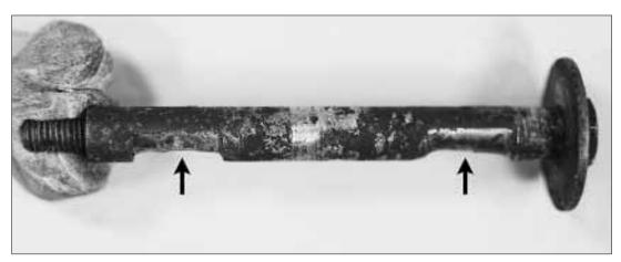
Figure 4. The worn pulley block securing bolt.
