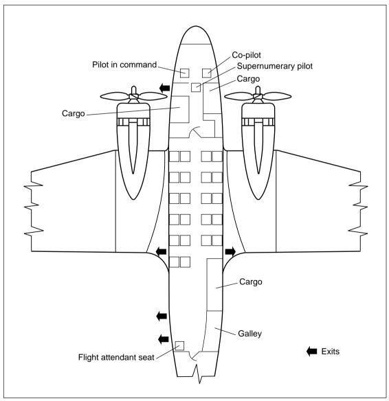
Figure 5. Diagram showing the internal layout of VH-EDC.
