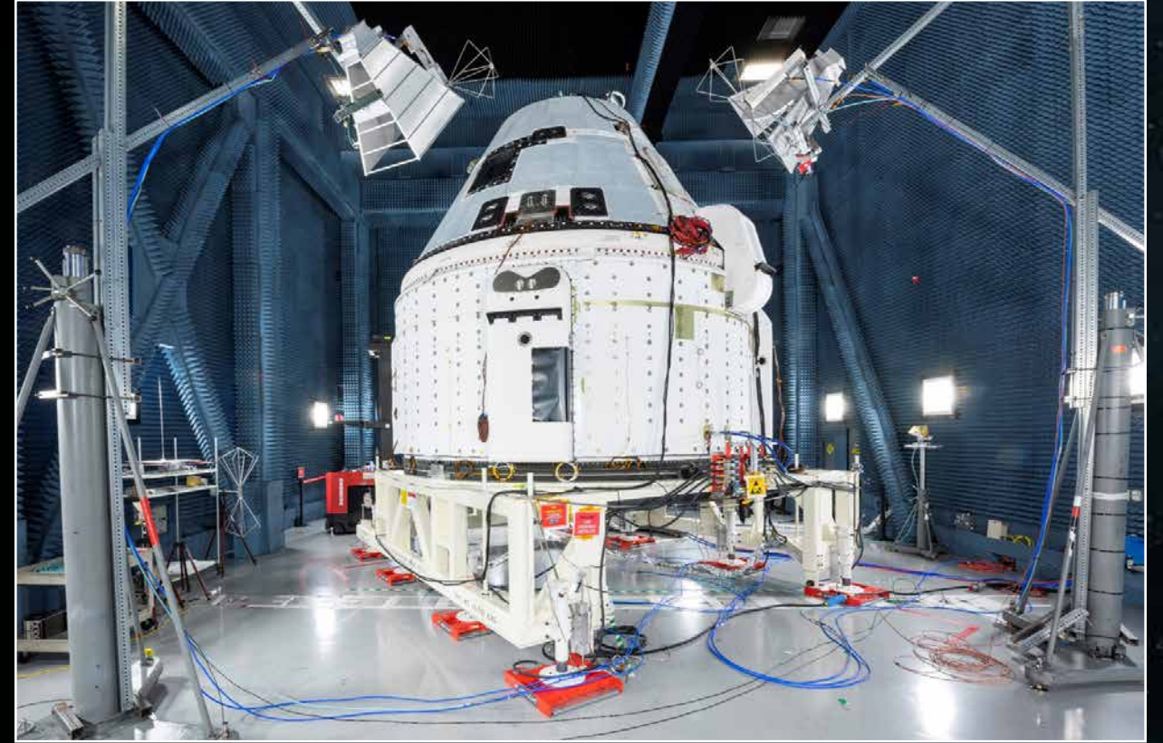
Boeing's CST-100 Starliner prepares for electromagnetic interference and electromagnetic contamination testing in a specialized test chamber at the company's Space Environment Test Facilities in El Segundo, California.
