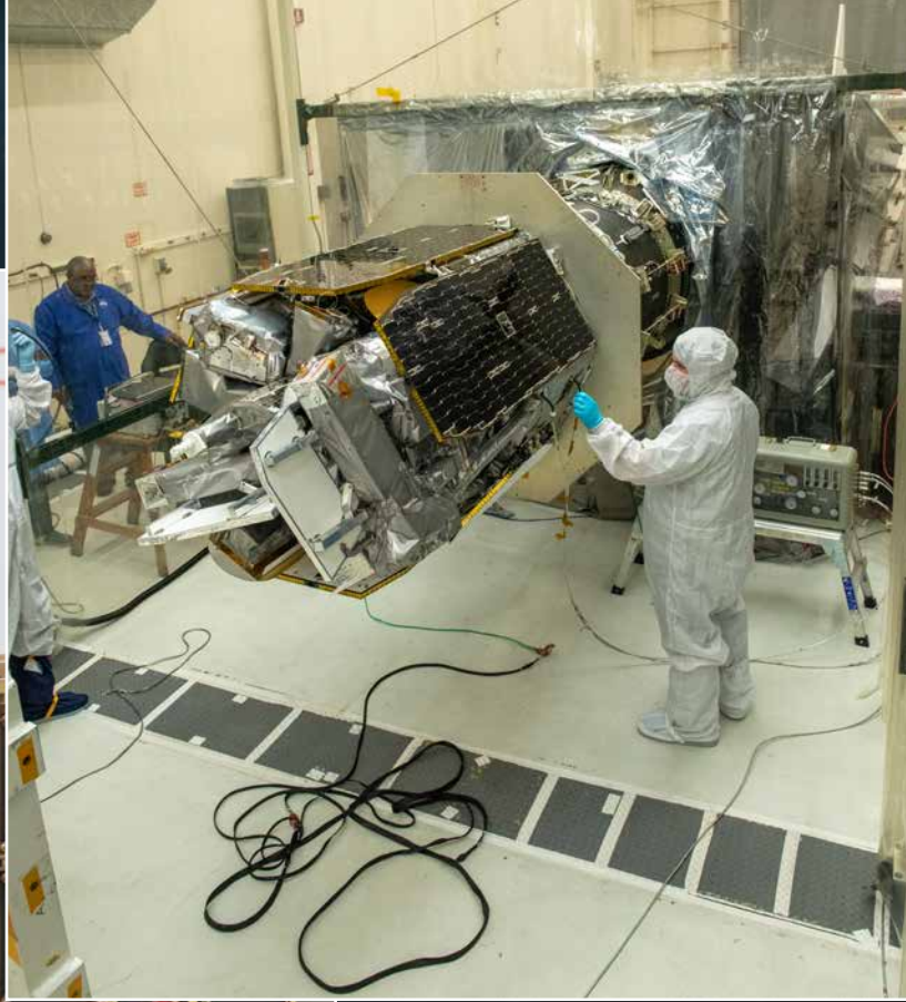
Above: Technicians attach NASA's ICON spacecraft to the Northrop Grumman Pegasus XL rocket at Vandenberg Air Force Base in California on Sept. 10, 2019.
