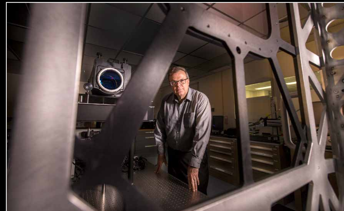
Mark Nurge, a physicist in Kennedy's Applied Physics Lab, stands near a laser interferometer, which is used to determine if there are acceptable levels of distortion and imperfections in windows. Nurge recently completed optical metrology testing and evaluation of all flight windows on the Orion capsule for Artemis I.
