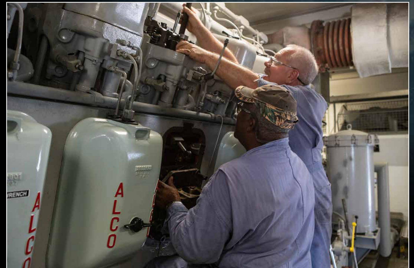
Below: Pat Brown, left, and William Vardaman, mechanical technicians with the Jacobs contracting team, perform engine maintenance on NASA's crawler-transporter 2 on March 26, 2019, in the crawler yard located in the Launch Complex 39 area.
