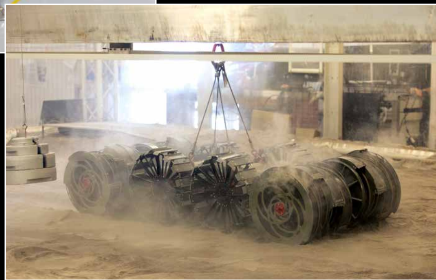
Above, the Restore-L payload undergoes preparations in the Space Station Processing Facility high bay. Managed by the agency's Goddard Space Flight Center in Greenbelt, Maryland, Restore-L is an in-flight robotic satellite servicer spacecraft. At right, the Granular Mechanics and Regolith Operations Lab tests the Regolith Advanced Surface Systems Operations Robot (RASSOR), a mining robot designed to extract usable elements from lunar regolith, undergoes testing in Kennedy's Swamp Works.
