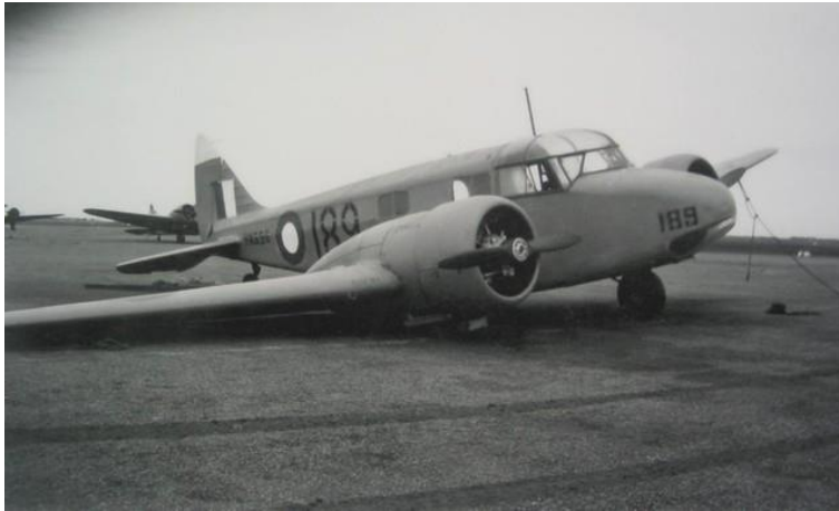
Oxford HN656 of No. 6 SFTS at Mallala with a collapsed right landing gear. Such accidents were common with both the Anson and Oxford fleet. (ADF Serials)
