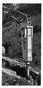
MONTABERT BRH 501 and BRH 250 Breakers have been successfully operating in Australia on excavators and backholes for more than 18 months. These Breakers have been used for secondary breaking in quarries, rock breaking in trenches and for foundations and for demolition.
