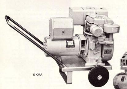
Powerlite LC models from 2KVA to 10KVA 1 & 3 Phase 240 or 415 volts. AC power. Adelux model with a current transformer control system for accurate voltage regulation. Ideal for electric motor starting. Carry frames STD equipment up to 4KVA trolly STD equipment from 5 to 10 KVA.
