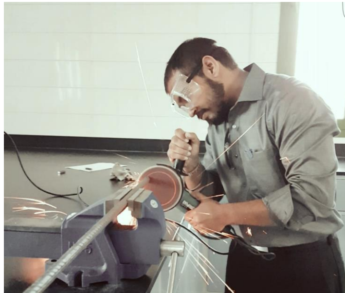
Figure 4.2.2 a – Grinding Operation prior Chemical Testing
