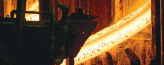
Billets from CC3 CC4 and CC5 are cut to  $3.8m \sim 12m$  by gas cutting equipment. A charge number is punched on each billet by a marking machine and dispatched for further processing to rolling mill for the production of rebar at Qatar Steel and QSC FZE, UAE. Billets are also sold to local and international customers.
