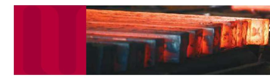
Continuous Casting is the process whereby molten steel is solidified into a "semi-finished" billet, boom, or slab for subsequent rolling in the finishing mills. Since its inception, a high degree of automation has enhanced operational excellence, increase in throughput by over 50% and reduction in cost.
