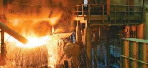
Qatar Steel was the first integrated steel plant in the gulf region that utilized a high percentage Direct Reduced Iron (95%) as a replacement of scrap for the production of steel from Electric Arc Furnaces. The original plant started in 1978 with an aim to utilize abundant natural gas resources available in Qatar for reduction of iron ore as the major feedstock for Electric Arc Furnaces.
