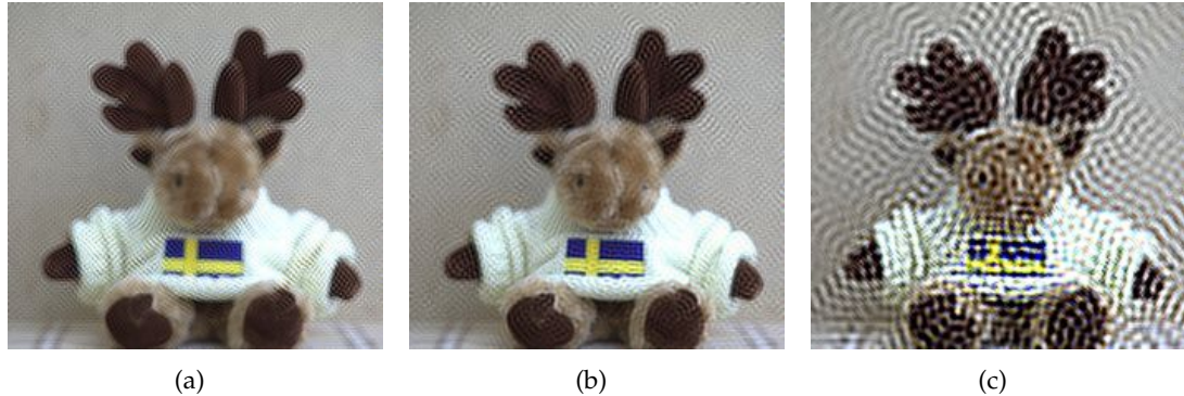
Figure 4.3: Propagation of artifacts in the image reconstruction method. The images the reconstruction of the image for three hypothesis-planes: (a) Image restored with hypothesis plane in front of the object. (b) Image restored with hypothesis plane at the object. (c) Image reconstructed with hypothesis plane at the background.
