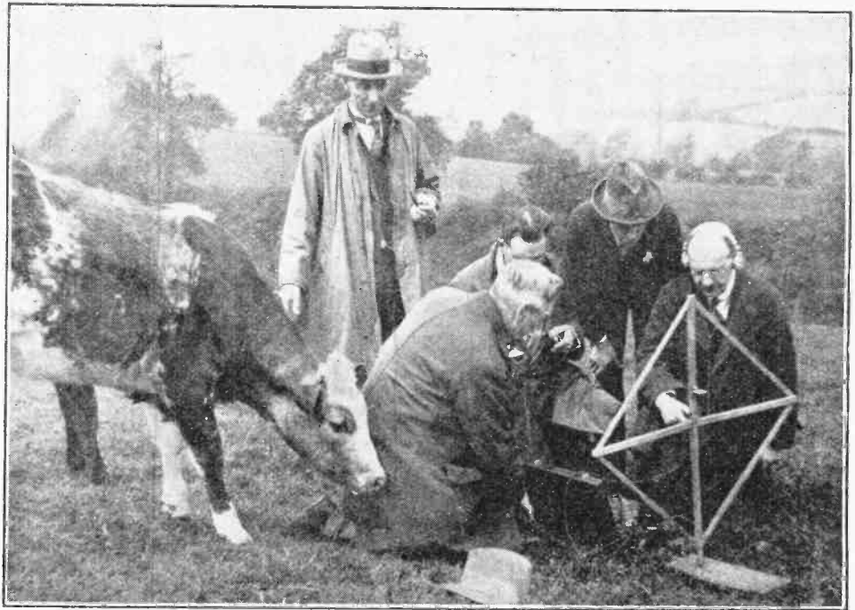
ON THE SCENT. A search party taking bearings on C.W. signals from the concealed station. The experiments obviously appealed to the bovine intelligence.
