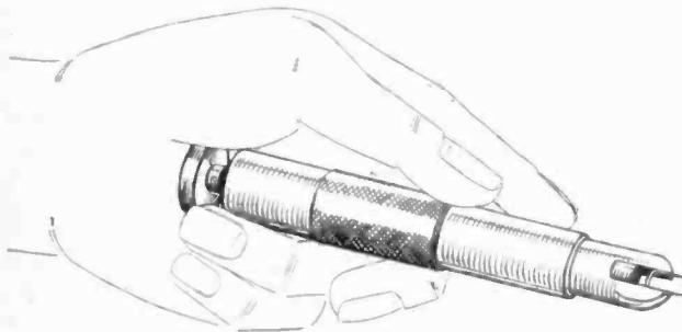
The Marple staple driver, an indispensable tool for stapling wires in positions normally inaccessible when driving the staple by means of a hammer.
