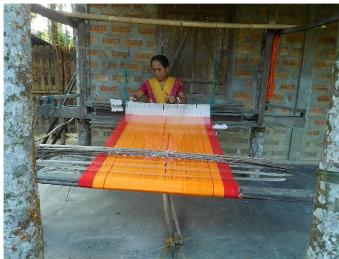
Figure 3. Weaving in throw shuttle loom.
