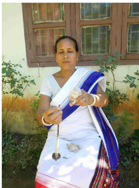
Figure 1. Eri yarn spinning with spindle.
