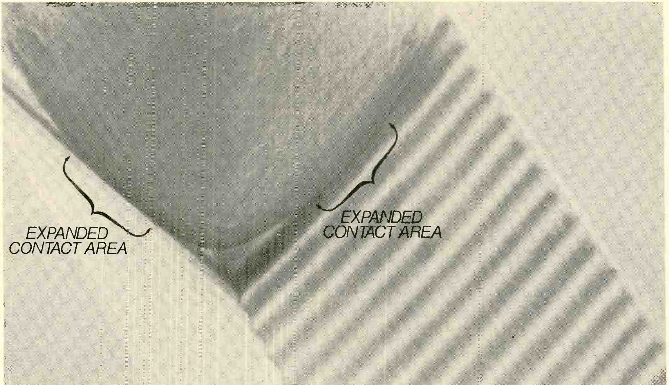
Scanning Electron Beam Microscope photo of Stereohedron stylus; 2000 times magnification. Brackets point out wider contact area.
