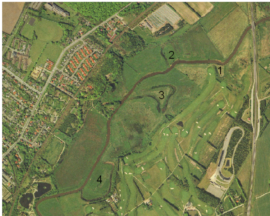
Aerial photograph of the project area prior to re-meandering of the river Varde. The location of former meanders 1–4 is indicated.
