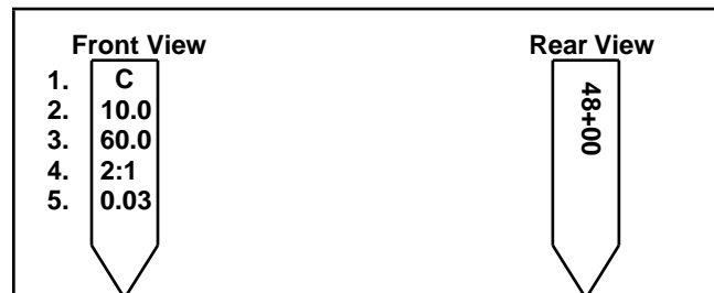
Figure 13-10: Station Numbering on Slope Stake.
