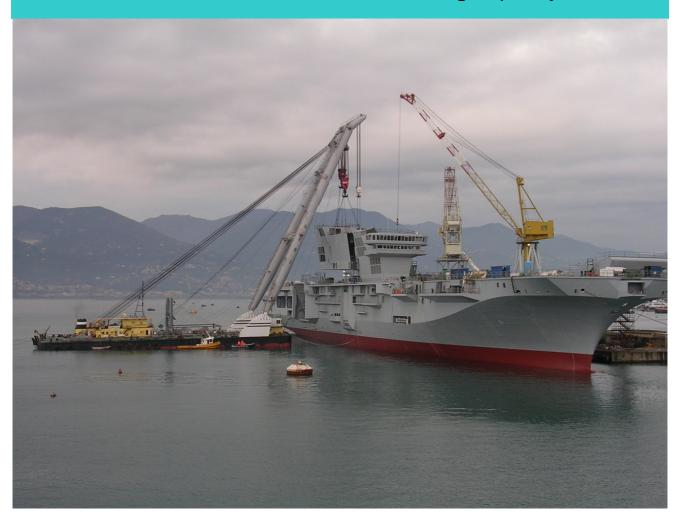
La Spezia (Italy)-FINCANTIERI Shipyards lifting accommodation structure (800 tons) on board the Italian Navy Aircraft Carrier "CAVOUR"
