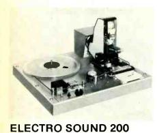
(shown here mounted on **Electro Sound** 100-48C tape winder for cassette operation.)
