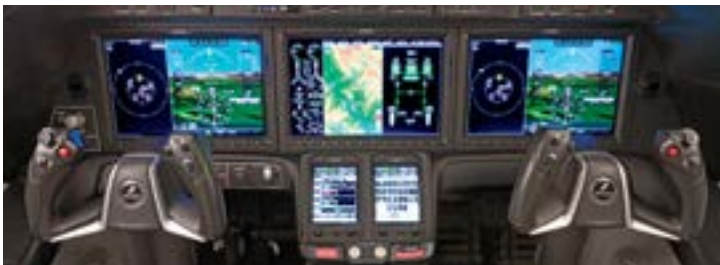
Location of the G3000's touchscreens relative to the pilot was a key concern for HondaJet designers, who wanted to find the optimal location and tilt angle to work eye-distance constraints. Avionics options include synthetic vision, radar altimeter, CPDLC, Iridium satcom, Tcas II, Taws A and Garmin SurfaceWatch.
