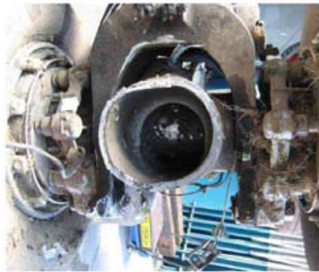
3. Shock Strut / Retract Arm Jams on and destroys upper part of inboard Trunnion Support Fitting
