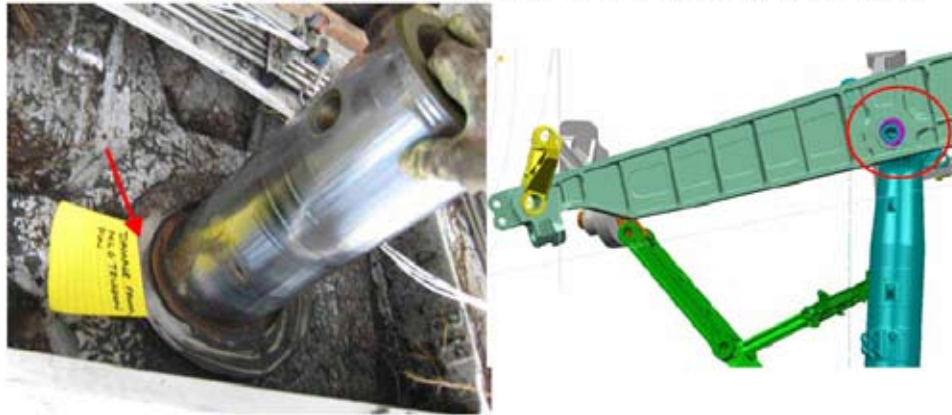
Gear Beam forced Inboard, reaches rotation limit and drives through swing link
