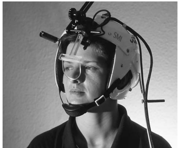
One, monitors the position of the eyes and head as a person scans a computer screen or the environment.
