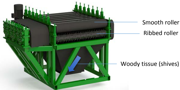
Figure 17: Example of breaking machine used in the decortication process
