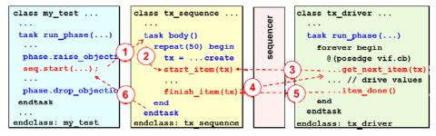
Figure 3 – Test/sequence/driver handshaking
