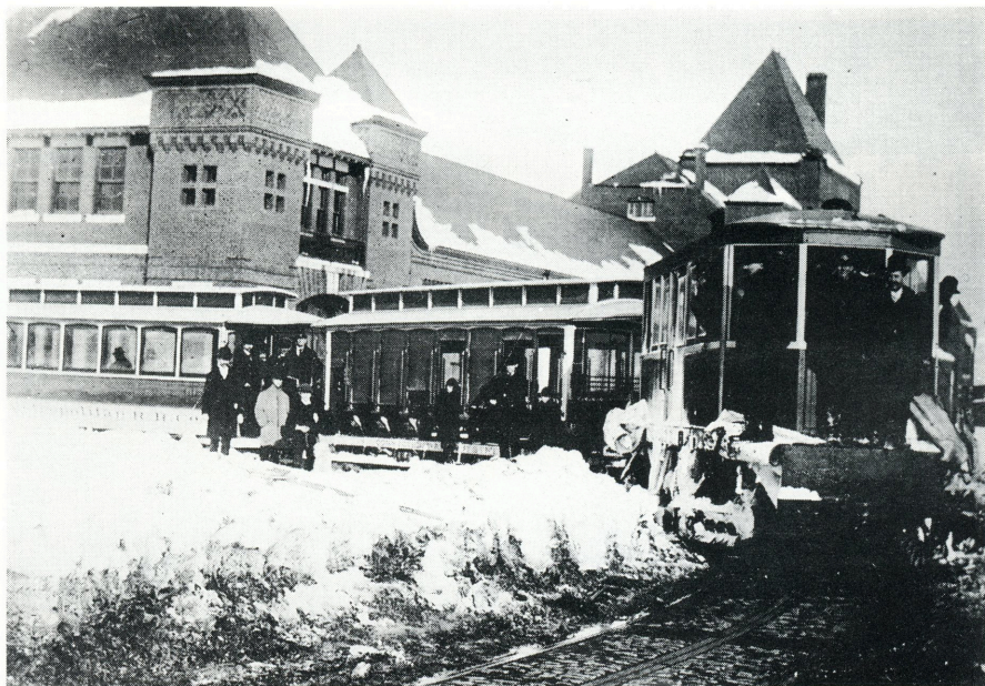
Metropolitan Railroad snow sweeper with a two-car train posed at Lincoln Park (Eastern) car house. Below the platform on which the men are standing is the rotating broom.
