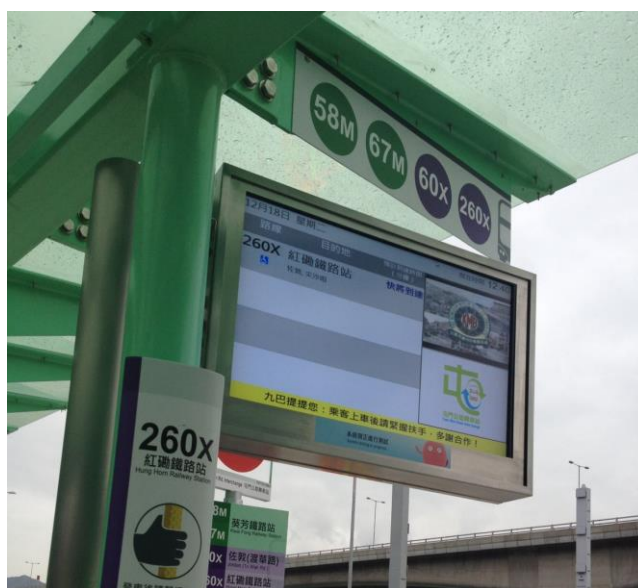
Figure 3C: Estimated bus arrival time system at Tuen Mun Road BBI
