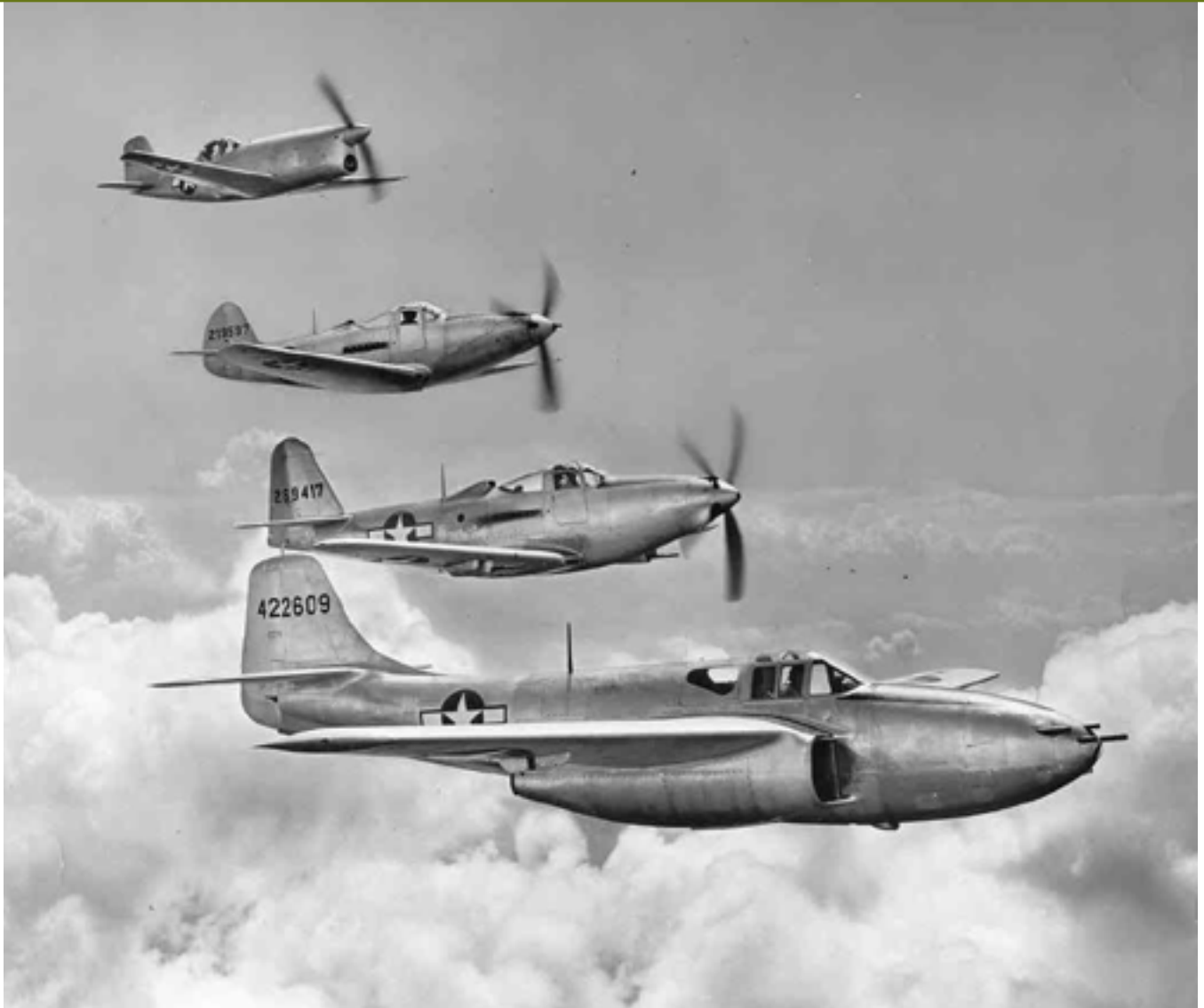
From top to bottom: An XP-77, an experimental fighter made of wood; a P-39; a P-63; and a P-59A – America's first jet fighter.
