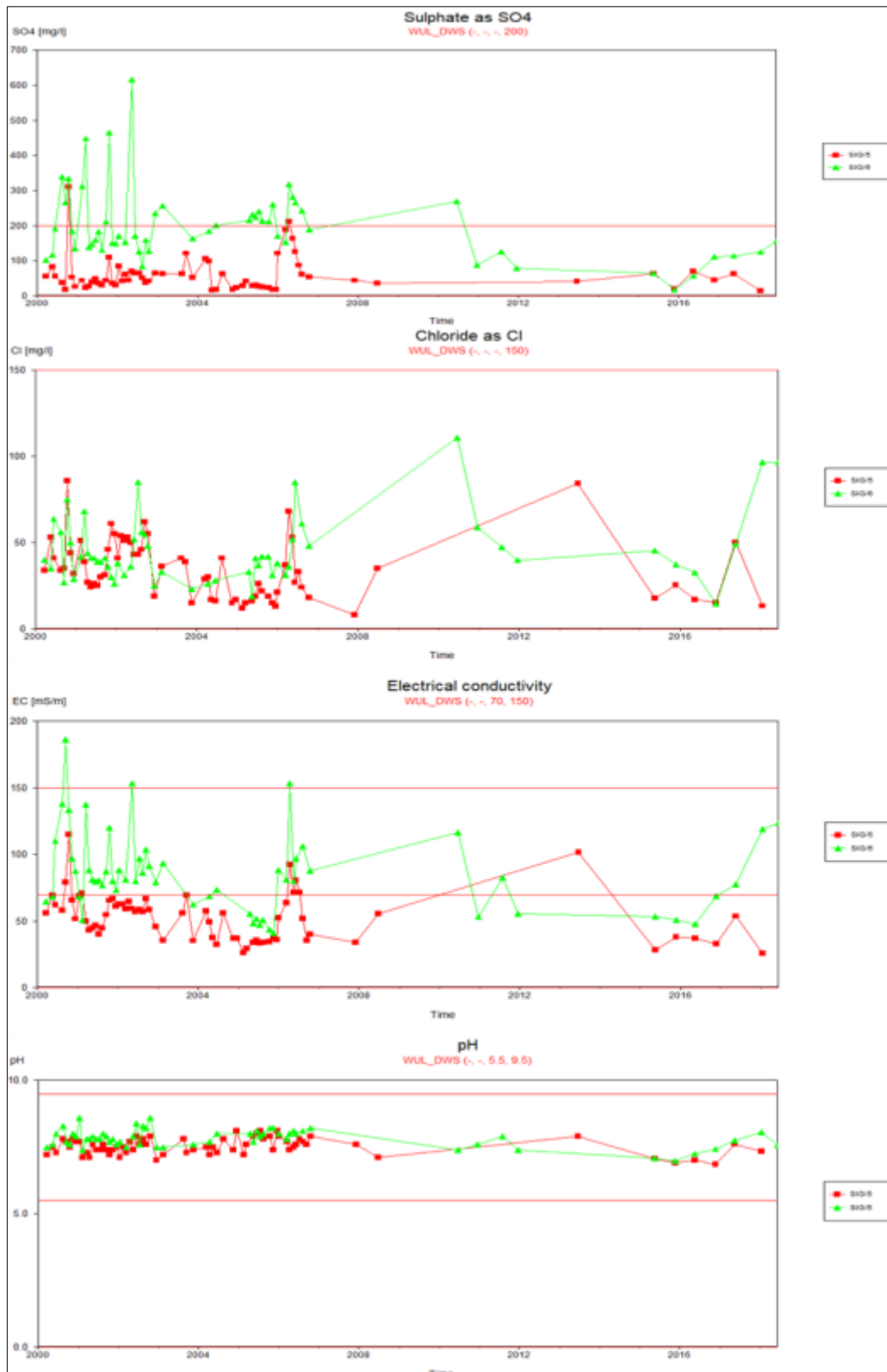
Figure 7-8: Electrical conductivity, pH, chloride and sulphate time graphs for the Leeuspruit tributary (SIG/5 & SIG/6) (IGS, 2018)
