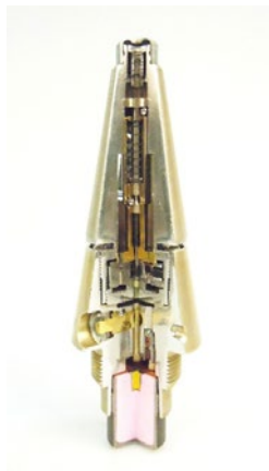
Left, MRV fuze. Right, MRV-U fuze cutaway. Image © Dutch EOD Center.
