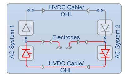
Figure 11: Bipole in Monopole Operation (Source: Alstom)
