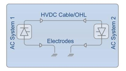
Figure 10: Monopole Configuration with Electrode Return (Source: Alstom)
