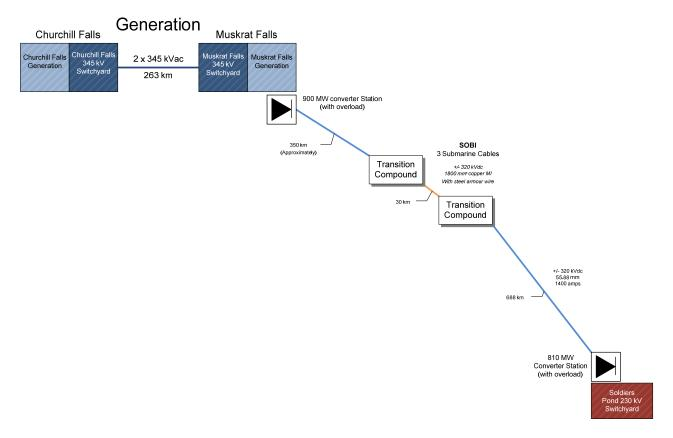
Figure 9: Labrador-Island Link HVdc System Configuration
