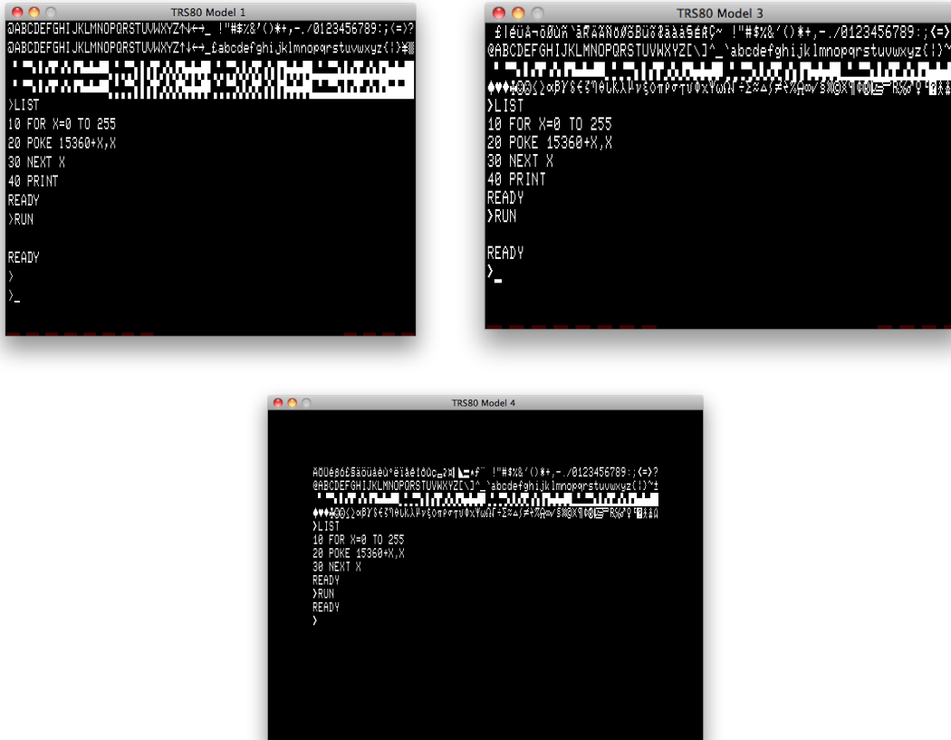
Figure 18. Character dumps for the TRS-80 Model I (top left), Model III (top right), and Model 4 (bottom), shown with generating BASIC programs on Macintosh-based emulators.
