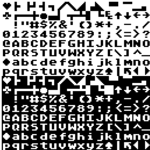
Figure 5. Character dump of ATASCII for the Atari 8-bit family (400, 800, XL, XE), showing both inverse and normal video.
