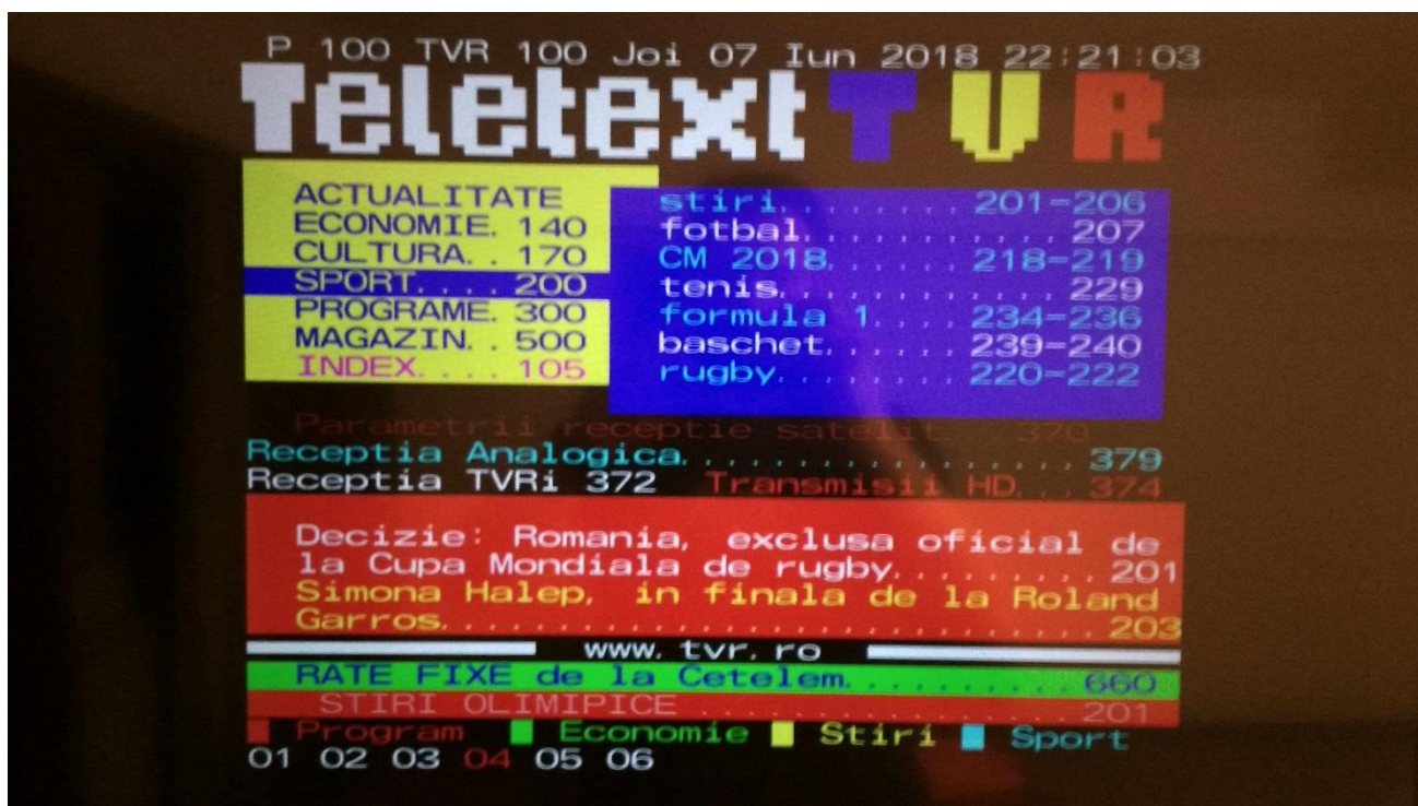
Figure 27. A present-day example of digital teletext in Romania, using block semigraphics from the teletext character set. (Ricardo Bánffy)
