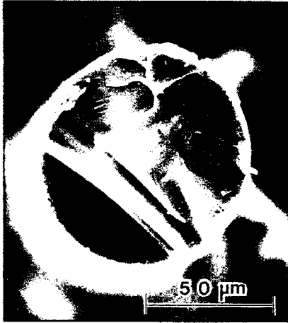
Co-investigators from NRL's Condensed Matter and Radiation Sciences Division and from the Carnegie Institute of Washington for the first time obtained useful X ray structure data from single crystals with submicrometer dimensions. Shown here is the end of a glass fiber with a fine Bi core. Scanning electron micrographs show cross section of the glass-enshrouded filament (left) and closeup of the bismuth (right). The ultrathin bismuth filaments were made by a researcher in the Materials Science and Technology Division.
