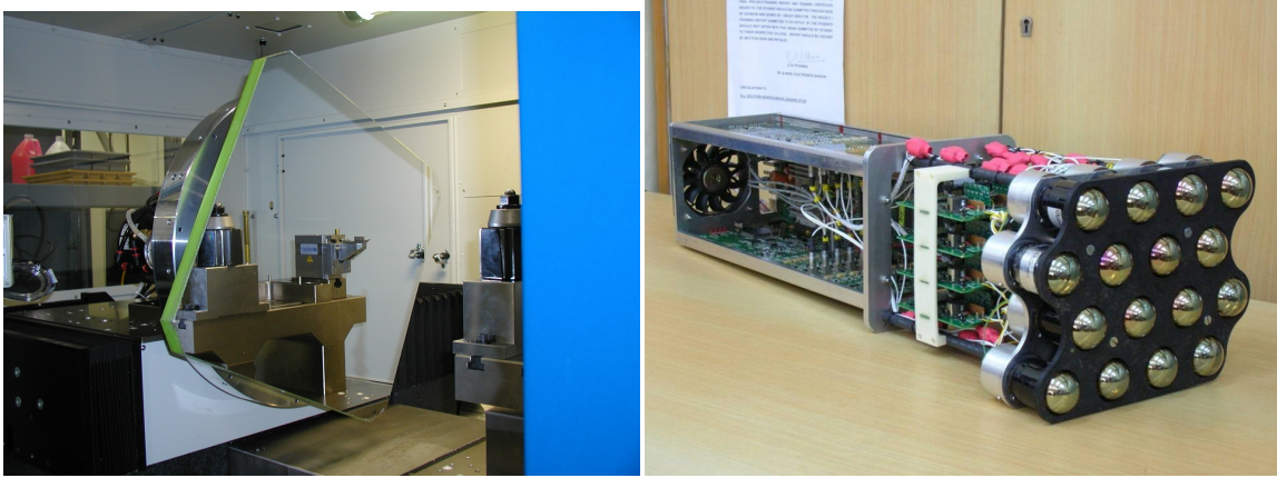
Figure 1: Left: A diamond turned mirror facet for the MACE light collector. Right: 16-channel camera integrated module for the camera of MACE telescope.
