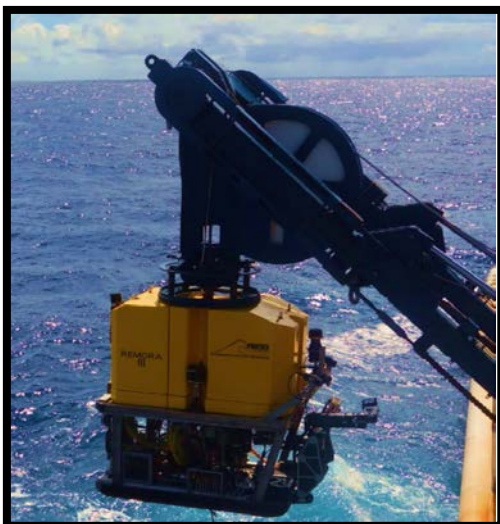
Figure 5. Remora III remotely operated vehicle.
