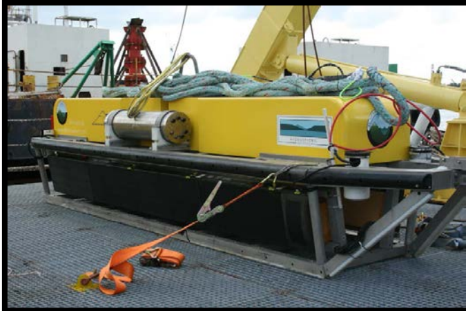
Figure 4. ProSAS SLH PS-60 deep tow vehicle
