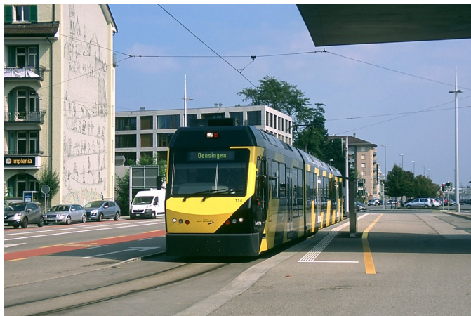
The ASm's single track terminal directly in front of the Luzernstrasse entrance to the Solothurn railway station. Note the height of the platform for the low-floor interurbans.
