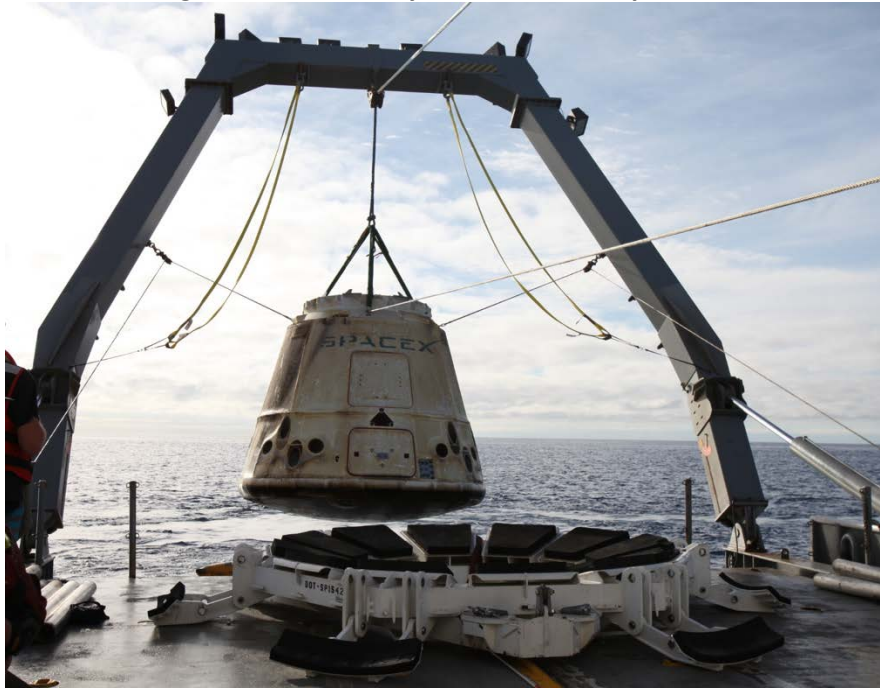
Figure 2-17. Recovery A-frame Crane Operation
