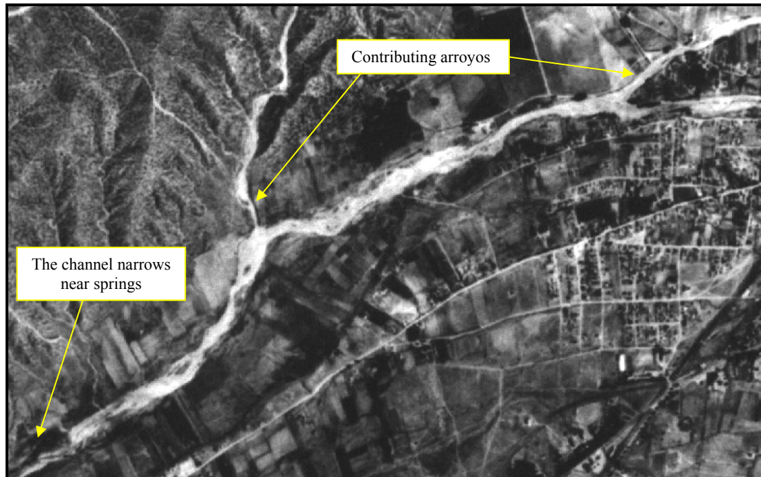
Figure 6.O. Braided channel configuration with contributing arroyos, 1936 Source: USDA Forest Service (2005)
