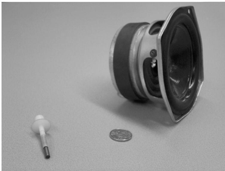
Figure 6.3-10. Left: the magnet system of the BaryBass transducer; right: a normal medium-sized bass loudspeaker. A 50 euro cents coin is shown for size comparison; the actual price is much less.
