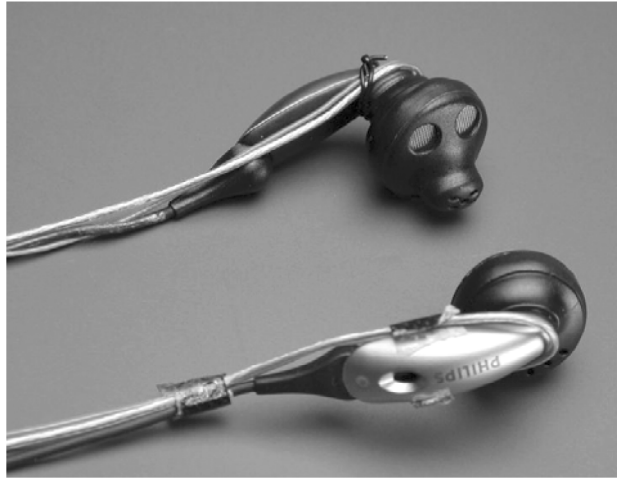
Figure 6.3-9. Prototype of earphones with integrated microphones.
