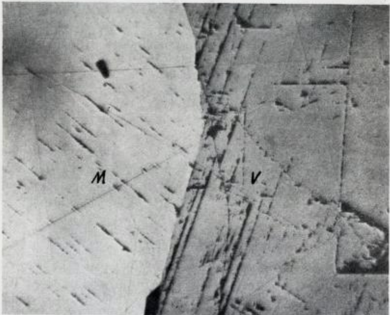
Fig. 8. Ore, Flåt mine. Millerite (M) and violarite (V). Pol. sec. ord. light 500 \times .
