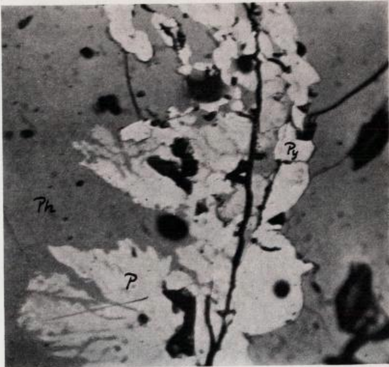
Fig. 6. Ore, Flåt mine. Pyrite and blades of pentlandite (P) in pyrrhotite (Ph). Pol. sec. ord. light 500 \times .
