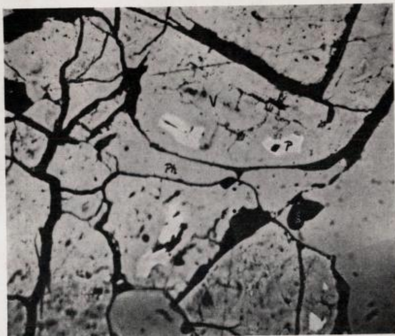
Fig. 10. Ore, Molland. Pyrrhotite with violarite and rests of pentlandite (P). Pol. sec. ord. light 500 \times .
