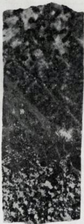
Fig. 11. Polished sections of a drill core showing the border between ore and silicate rock in the hanging wall of the ore body. Flåt mine. 2 ×.
