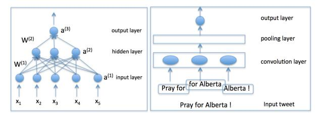
Figure 1. Fully connected neural network (left hand side); Convolutional Neural Network (right hand side).
